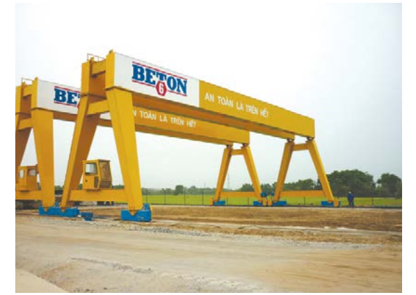
Cồng trục / Gantry Crane Quatity: 34 units Capacity: 3 - 50 tons
