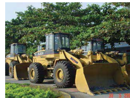
Xe xúc lật / Wheel Loader Quantity: 09 units Capacity: 2.5 - 3 m³
